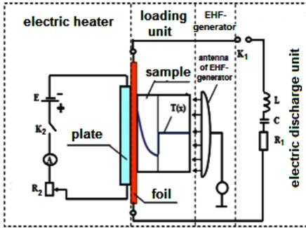
**Figure 6.** Sample combined heating experiment scheme
