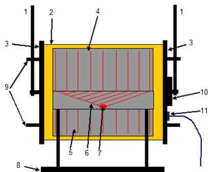
**Figure 9.** Bench scheme (front view): 1 is pendulum suspension; 2 is test cylindrical shell; 3 hermetic lids; 4 is explosive device of distributed impulse loading, upper part; 5 is explosive device, lower part; 6 is detonation wiring; 7 is initiation point; 8 is explosive loading device stand; 9 are stoppers; 10 is spring rotary mechanism; 11 is sealed feed-through
