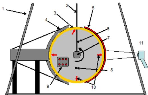
**Figure 8.** Bench scheme (side view): 1 is pendulum post (top hinge is not shown); 2 is pendulum suspension; 3 is test cylindrical shell with lids; 4 is explosive device (CCI or ESC) located on the stand; 5 is pyrotechnic composition or TEH; 6 is detachable stopper; 7 is spring rotary mechanism; 8 is non-detachable stopper; 9 is sealed feed-through; 10 is locations of strain gauges; 11 is optical pyrometer
