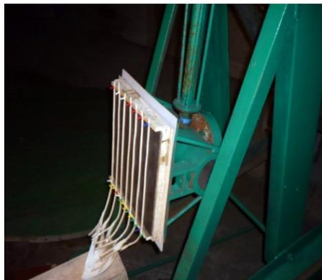
**Figure 1.** Tape explosive charge
