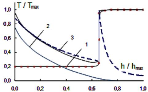
**Figure 7.** Temperature profiles in the case of combined heating of a two-layer composite plate: 1 is EHF-heating; 2 is electric heating; 3 is total heating; dashed line is simulated profile
