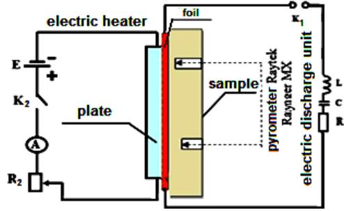
**Figure 3.** Scheme of testing plate
