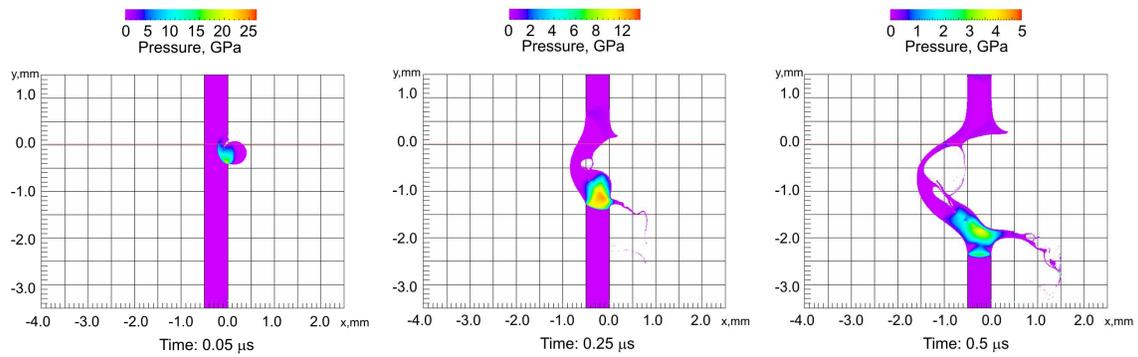
**FIGURE 4.** 2D-pressure field for 30 degrees impact angle 4 km/s velocity penetration, at 0.05  $\mu$ s, 0.25  $\mu$ s and 0.5  $\mu$ s.
