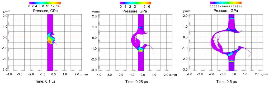
**FIGURE 2.** 2D-pressure field for 60 degrees impact angle 4 km/s velocity penetration, at 0.1  $\mu$ s, 0.25  $\mu$ s and 0.5  $\mu$ s.
