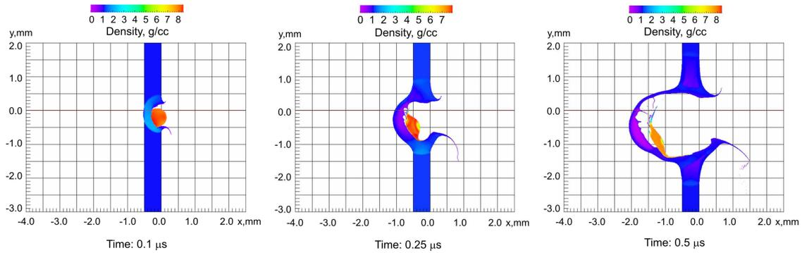
**FIGURE 3.** 2D-density field for 60 degrees impact angle 4 km/s velocity penetration, at 0.1  $\mu$ s, 0.25  $\mu$ s and 0.5  $\mu$ s.
