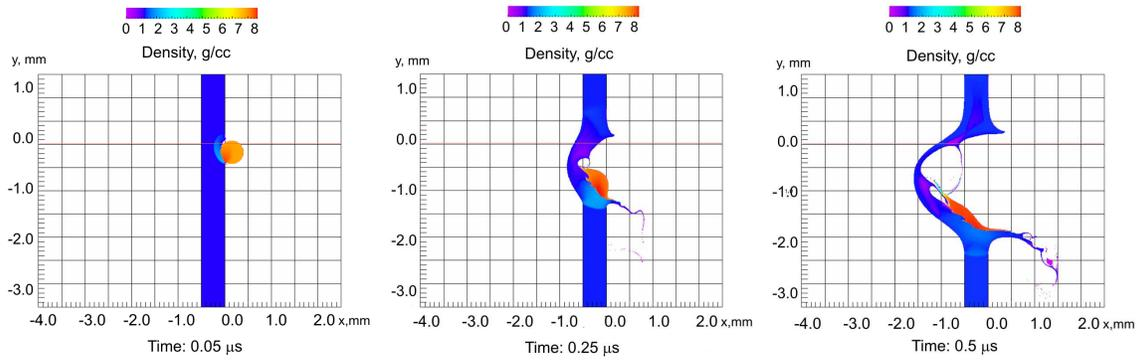
**FIGURE 5.** 2D-density field for 30 degrees impact angle 4 km/s velocity penetration, at 0.05  $\mu$ s, 0.25  $\mu$ s and 0.5  $\mu$ s.
