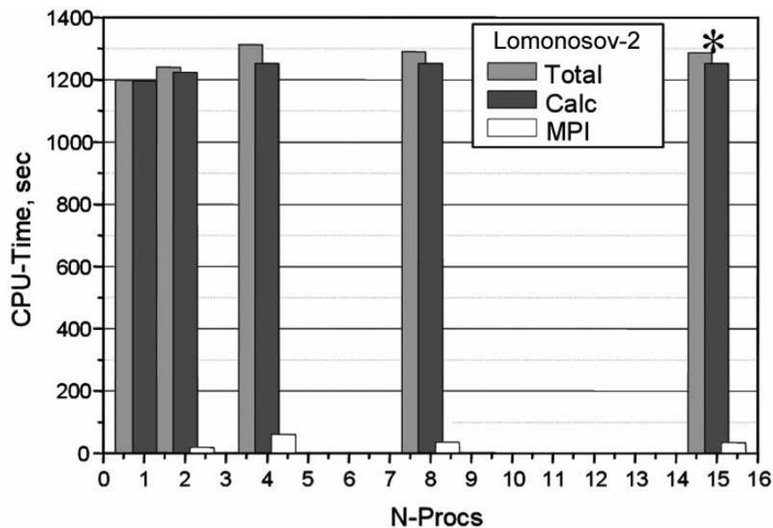
FIGURE 1. Parallel CPU-time profiling results on Lomonosov-2 supercomputer at MSU.
