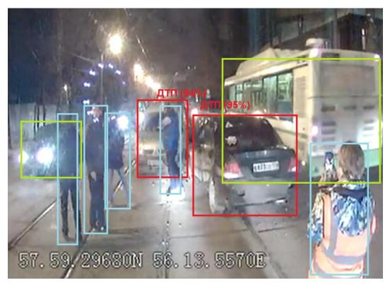
Fig. 3. An example of an accident detector on board of the passenger bus
